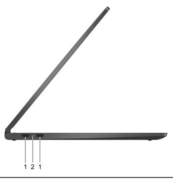
1. Power connector/USB-C<sup>TM</sup> connector (2)
